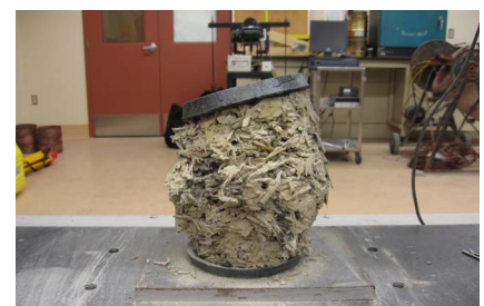
Figure 2: Tested hempcrete cylinder
