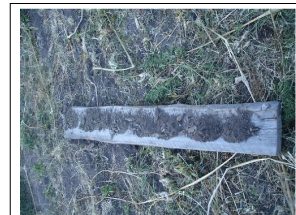
Site I. Second core from right has non-permeable layer preventing proper root development
