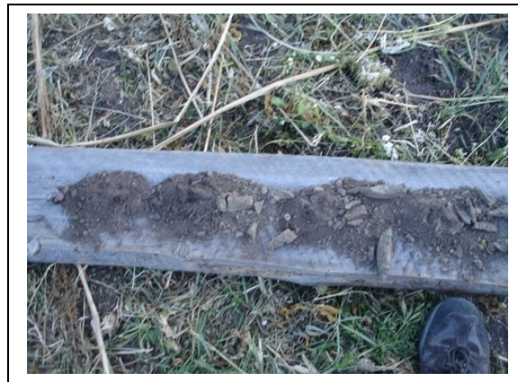
Site I. Detailed picture showing root development issue with non-permeable layer. (Second core from left)
